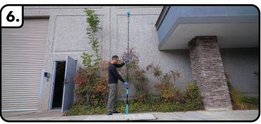
Extend (or retract) pole to desired height (only when pole is vertical).
