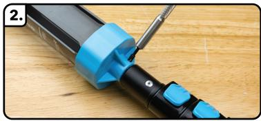
Place supplied grub screw in the small hole in the base and tighten.
