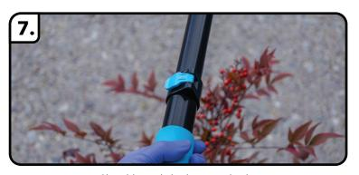
Close blue pole latches completely (to avoid pole collapse when in use).
