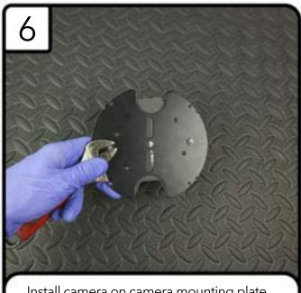
Install camera on camera mounting plate
