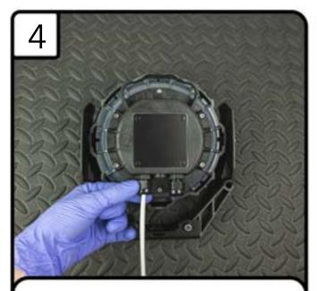
Insert power/data cables and tighten down cable gland cap
